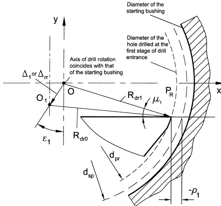
Fig. 1. Geometrical model to calculate the diameter of the hole after the first stage of drill entrance when there is no misalignment.
