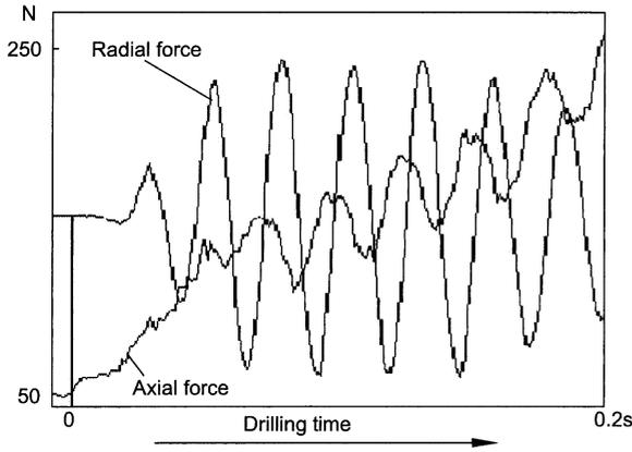
Fig. 4. Superimposed trace of axial and radial forces showing their phase relation.
