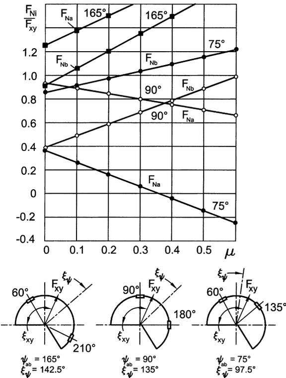
Fig. 7. The relationship  $F_{Ni}/F_{xy} = f(\mu)$  for different locations of the supporting pads.
