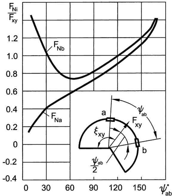
Fig. 6. The relationship  $F_{Ni}/F_{xy} = f(\psi)$  under symmetrical location of the supporting pads relative to the resultant force  $F_{xy}$ .
