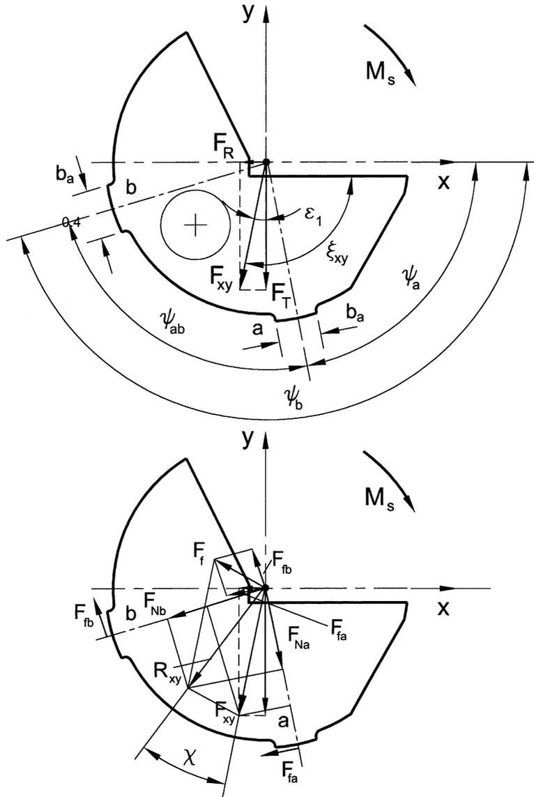
Fig. 5. Model of forces acting on the gundrill.
