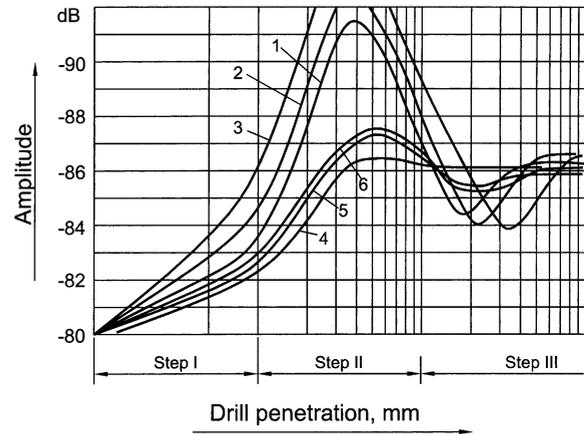
Fig. 3. Comparison of the intensity of transverse vibrations at the drill entrance for a gundrill with the supporting continuum (curve 1–3) (Star Cutter Co.) and that with two supporting pad (curves 4–6) (ASTVIK 15-03-02 design by Hyper Tool Co.). Gundrills of 8 mm dia., workpiece material—aluminum alloy 316. Curves 1,4—5800 rpm, 710 mm/min; 2,5—6800 rpm, 850 mm/min, 3,6—8000 rpm, 1060 mm/min.
