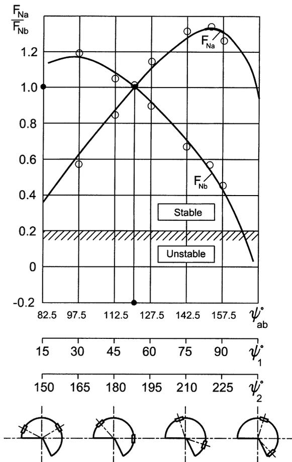
Fig. 9. Finding the optimum location angles of the supporting pads under given  $\psi_{ab} = 135^\circ$ ,  $\mu = 0.15$ . Experimental points are shown for ASTVIK 15-03-02 design by Hyper Tool Co. Gundrilling regime was: rotation speed 6800 rpm, feed rate 850 mm/min, cutting fluid flow rate 12 l/min.
